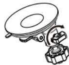
b. Please clean up the windshield (inside), put the holder in front of rear mirror, and then press the lever down to ensure the holder was fixed well.
