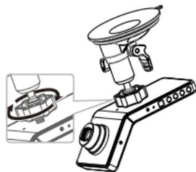
\* Left turn the knob of suction cup holder to adjust the lens angle and right turn to fix it.
