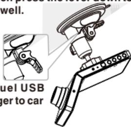
c. Use the USB cable of Duel USB Charger to connect car charger to car socket.
